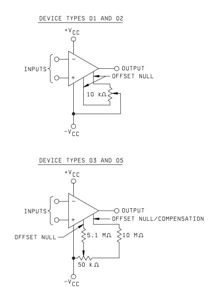
FIGURE 2. Offset null circuits.
